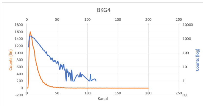
Figure 8: BKG4 was performed after both BKG1-2 and SR1-2 to see if the background light changed during the study. This was the first one to be performed after the voltage was turned back on. The intensity detected was slightly higher than former ones.
